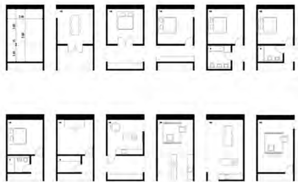
Figure 1: Functional module measuring 22m 2 adapting to the different functionalities of the accommodation
